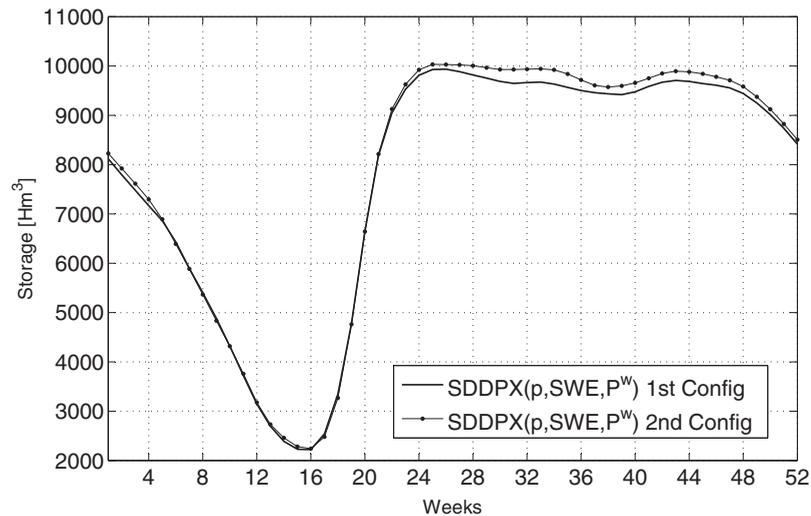
**Figure 5.** Average weekly storages at reservoirs Passes-Dangereuses (RPD) and Lac-St-Jean (RLSJ)-Formulation SDDPX( $p, SWE, P^w$ ) for both configurations.
