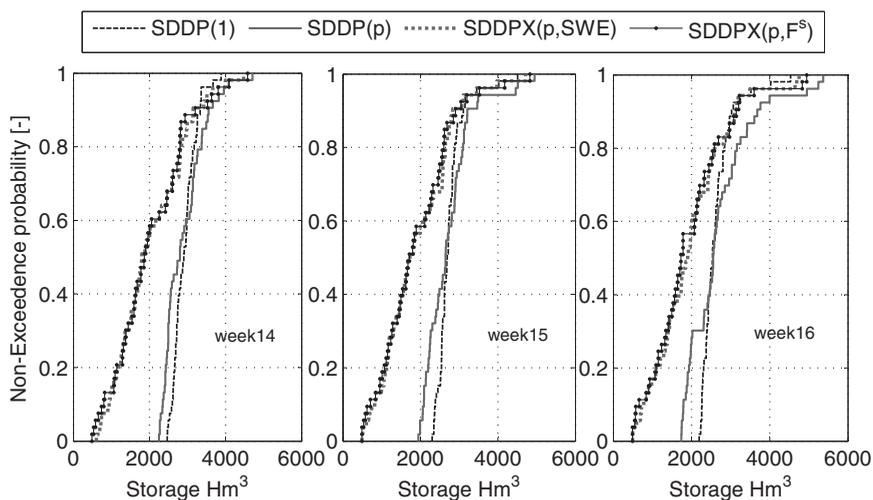
Figure 3. Statistical distribution of the accumulated storages for the largest reservoirs for weeks 14, 15, and 16. First configuration.
