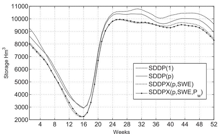
Figure 2. Weekly mean storage at reservoirs Passes-Dangereuses (RPD) and Lac-St-Jean (RLSJ). First configuration.
