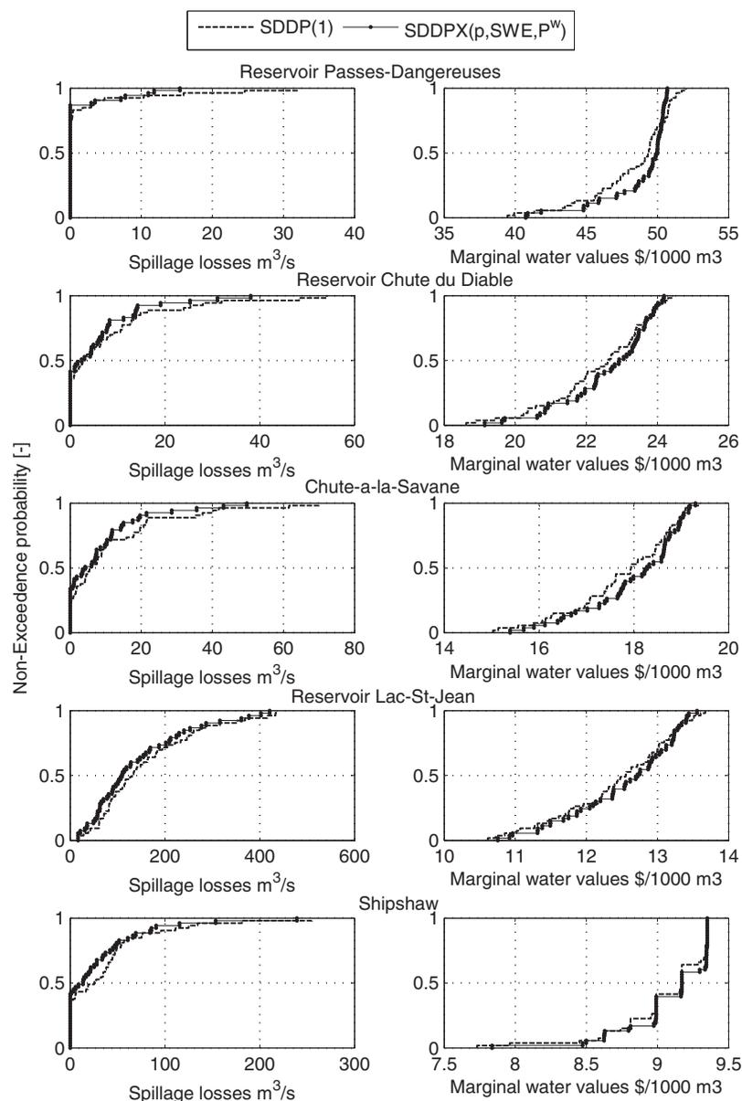
Figure 4. Statistical distributions of (left) spillage losses and (right) marginal water values. First configuration.
